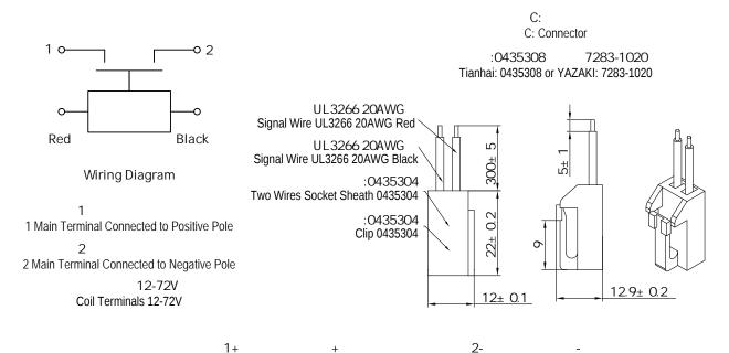
Note: The product main contact "1+" which is marked near the bolt is connected to the load "+" terminal, and "2-" is connected to the load "-" terminal.
